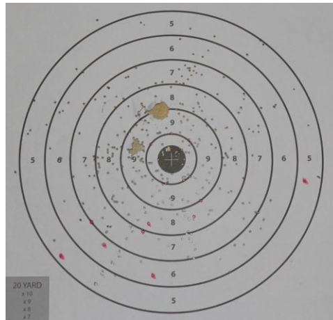
Figure 2: Target showing the spread of 12 gauge #7½ shotgun pellets.
