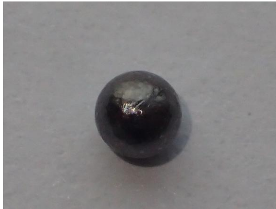
Figure 1: A 44× optical microscopy of an unfired 12 gauge #7½ shotgun pellet.
