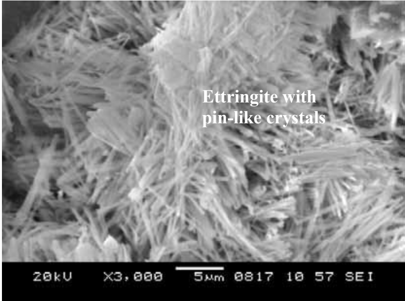
Fig. 6. SEM micrograph of CW5 subjected to 5 % MgSO 4 attack for 180 days
