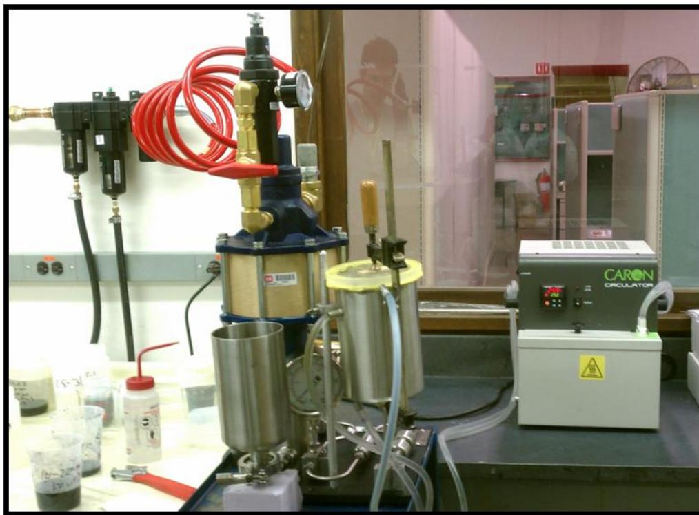
**Figure 1.** Modified M110-Y microfluidizer apparatus.
