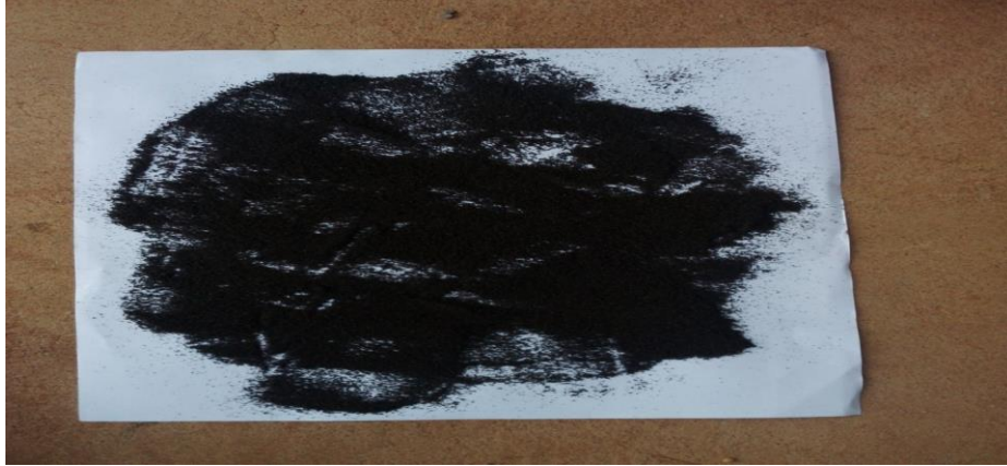
Figure 3: Iron particles (diameter 0.013mm) used for the experiment
