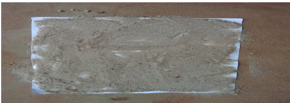
Figure 2: Silicon IV oxide (diameter 0.012mm) used in the experiment
