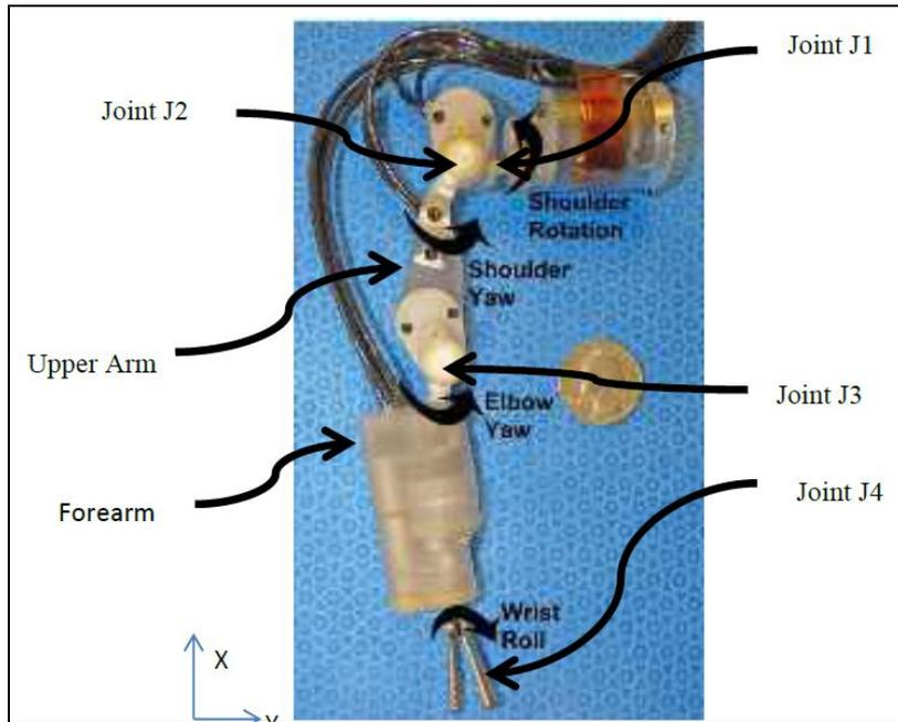
**Fig 2 Detail Design of the Robot**
