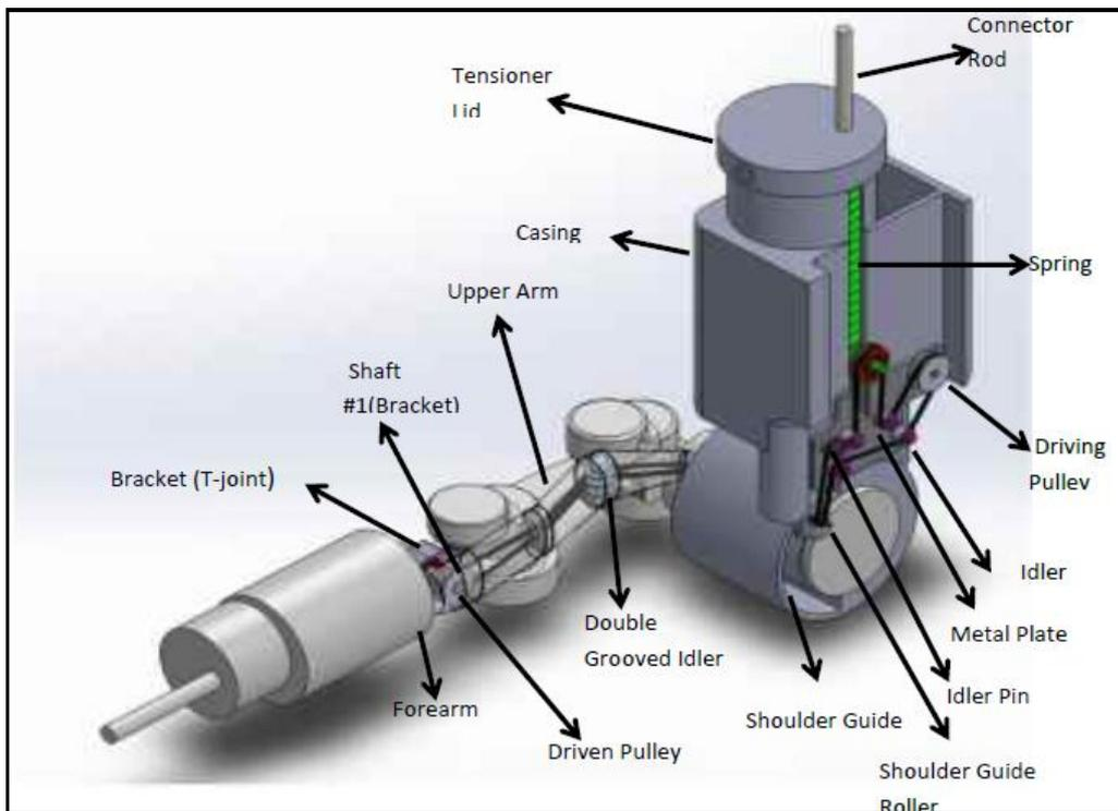
**Fig.3 entire assembly of the design system**
