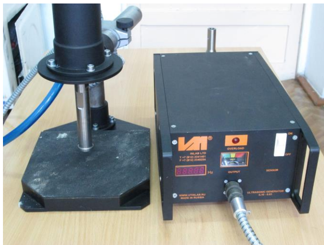
Figure 1. Experimental setup for the ultrasonication of silica nanopowders in water.
