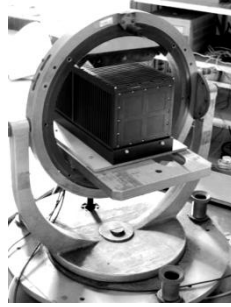
Figure 2. The system is fixed on the manual three-axis turntable
