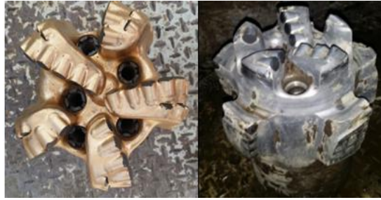
Figure 11. Comparison of drill bit with mud motor used (4158m ~4213m)
