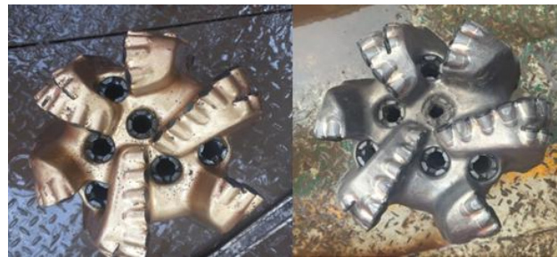
Figure 14. Comparison of drill bit with torkbuster used (4380m ~4444m)
