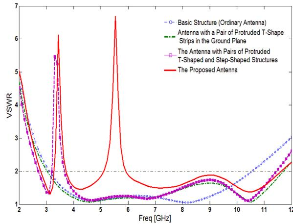
**Fig. 3 Simulated VSWR characteristics of the various structures of the presented antenna.**
