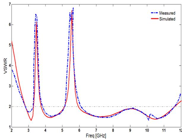
**Fig. 5 Measured and simulated VSWR characteristics of the proposed antenna**
