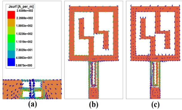
**Fig.4. Simulated surface current distributions for the proposed antenna (a) at the extra resonance frequency (10.5 GHz), (b) at the first notched frequency (3.5 GHz), and (c) at the second notched frequency (5.5 GHz)**
