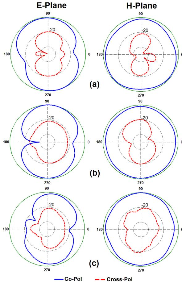
**Fig. 6 Measured radiation patterns of the proposed antenna at (a) 4.5 GHz, (b) 7.5 GHz, and (c) 10.5 GHz.**
