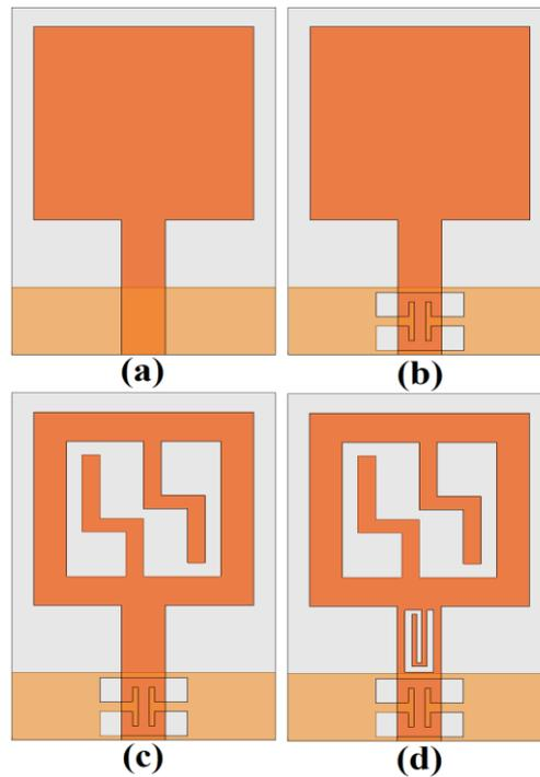
**Fig. 2** (a) Ordinary monopole antenna, (b) the antenna with a pair of T-shaped strips protruded inside the slot in the ground plane, (c) the square-ring antenna with pairs of protruded step-shaped and T-shaped strips, and (d) the proposed antenna structure
