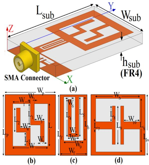
**Fig. 1** Geometry of proposed antenna (a) side view, (b) radiating patch, (c) feed-line, (d) modified ground plane
