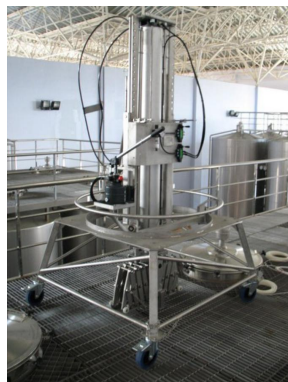
Figure 8. Machine that presses the cap into the mash of Château Junding in Yantai city
