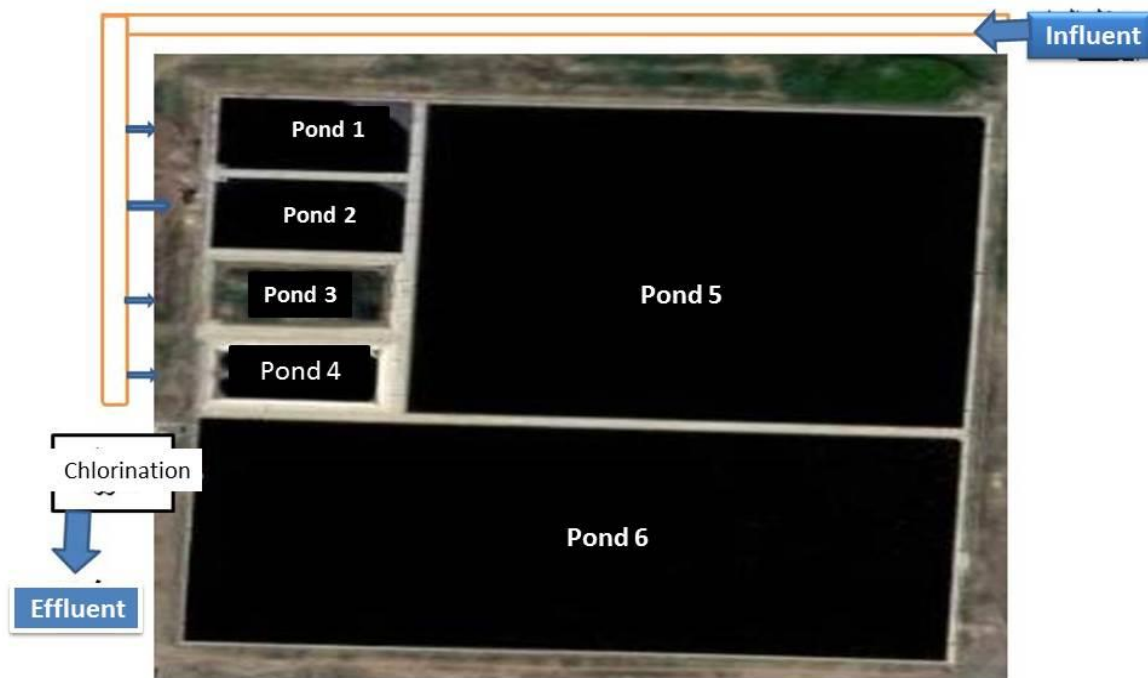
Figure 2. Design of the WWTPs components
