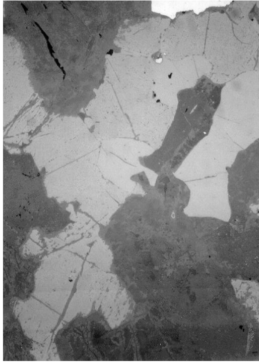
Figure 8. Photomicrograph of vanadium-rich sample from the Bell River Complex (Taner et al., 1998). This photo shows the relationship between cumulus silicate minerals and interstitial oxide minerals (medium gray magnetite and light grey ilmenite: reflected light, 1.8 mm field of view).
