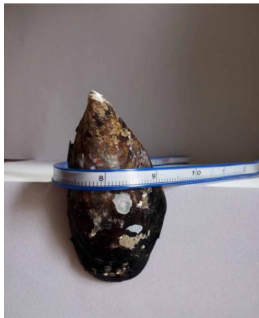
Fig.3. Measuring method of shell section curve
