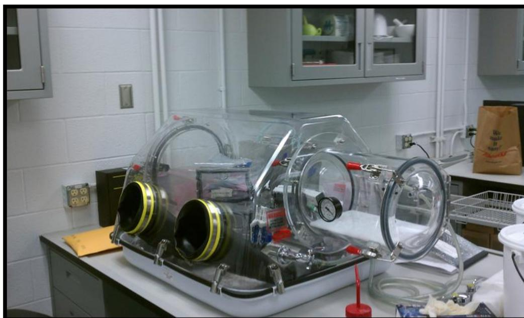
**Figure 2.** La Petite glove box used to safely load powder CNTs into resin.
