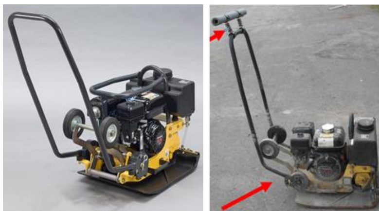
Fig. 3 View of vibration board before and after the modification
