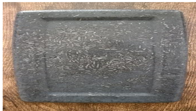
Fig 3. AA phantom simulating a human quadriceps (NaCl concentration = 7g/L; graphite concentration = 6g/100ml).
