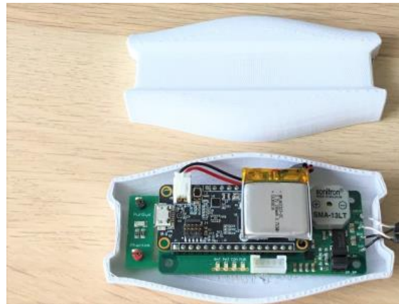
Fig 2. Electronic board of bioimpedance BioZ (Module Phi-Light, RunSys, France)
