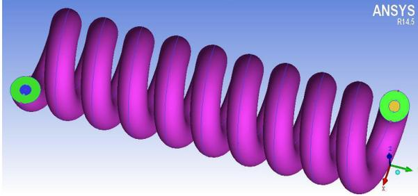
Fig.2 Geometry of EATHE model
