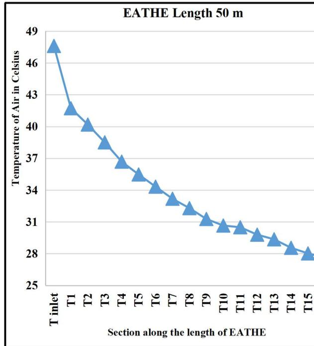
Figure 4.45 Graph of temperature v/s length for pipe length 50m of EATHE
