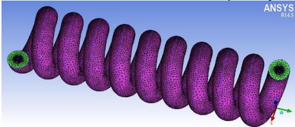
Fig. 3 Meshing of EATHE model
